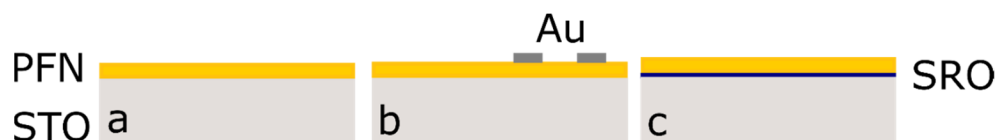
Figure 1. Different sample structures for the different measurements: (a) for XRD, RHEED, and UV-Vis; (b) for TLM; (c) for IPES/UPS.
