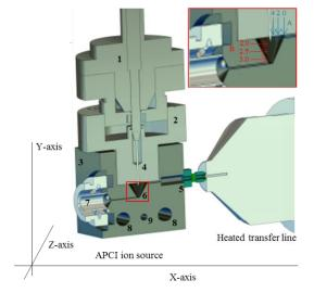
Side view of the prototype GC-APC-MS coupling with:1. Electrical supply2. Height adjustment3. Ion source body4. Corona needle
