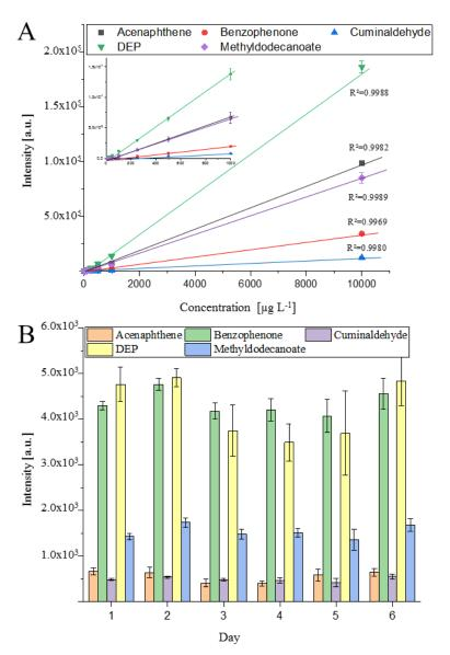
**Figure 4.** Performance of the prototype ion source. (**A**) shows the linearity and standard derivation of the standards between 10–10,000 µg L<sup>-1</sup>. Each concentration was analyzed three times (n = 3). (**B**) shows the repeatability of the measured values over six days with five injections (n = 5) at 1 mg L<sup>-1</sup> each day.
