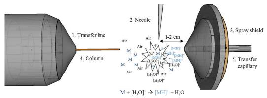
**Figure 1.** Overview of a conventional gas chromatography-atmospheric pressure chemical ionization-mass spectrometry (GC-APCI-MS) set up. The system contains the transfer line (1), the APCI corona needle (2), spray shield (3), the GC column (4), and a transfer capillary (5). The needle is mounted 1–2 cm from the interface system. Between the needle and the inlet system is the plasma zone, where the reaction cascade take place.
