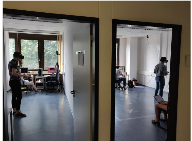
Fig. 3. In the remote setting, the tracking areas of both rooms were identical, by visualizing the dimensions of one room on the floor of the second room. In both conditions, each HMD requires to be operated on individual PCs. The synchronization of the game is done via a broadband local area network.
