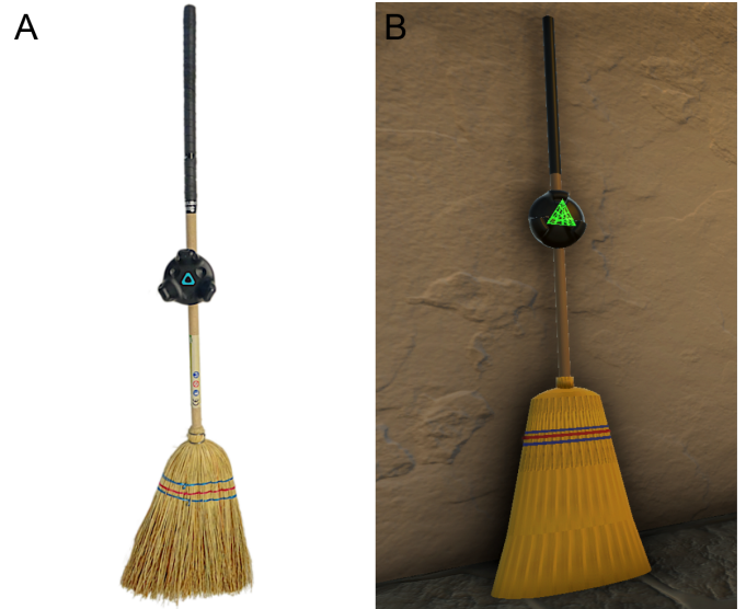
Fig. 1. A The real world broom has a length of 135 centimeters. An HTC Vive tracker is attached to the broom using a clamp. In total the broom weighs 594 grams. B The virtual broom has the same dimensions as the real one. A virtual tracker model is attached to the broom and acts as a visual indicator displaying whether the energy shock can be used (green light vs. red light).
