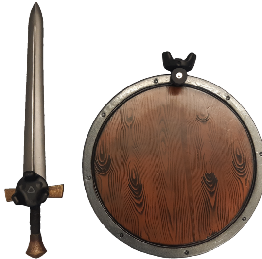
FIGURE 7.2: The sword is 16 cm wide, 71 cm long, and weighs 356 g, including the HTC Vive Tracker. The shield is 50 cm in diameter and weighs 829 g, with the mount and HTC Vive Tracker included. While the sword is held in hand, the back of the shield has a mount for the entire forearm. ©2021 IEEE
