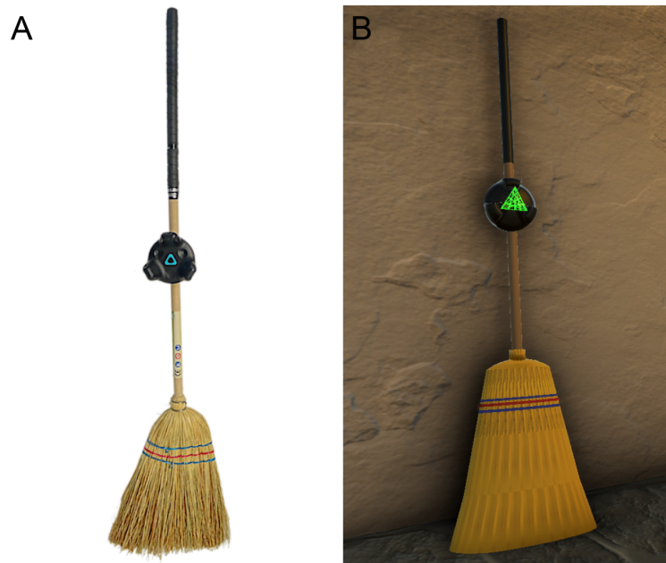
FIGURE 4.1: (A) shows the real broom used as a controller for Ghost Sweeper. (B) shows the virtual broom counterpart in Ghost Sweeper. ©2020 IEEE
