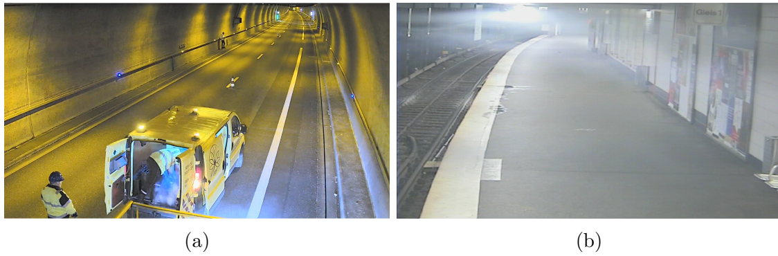
Figure 5.21: Typical global light changes in semi-outdoor scenarios, which lead to challenging smoke detection. (a) Blinking lights during smoke event in a tunnel. (b) Headlights of an arriving train behind smoke.
