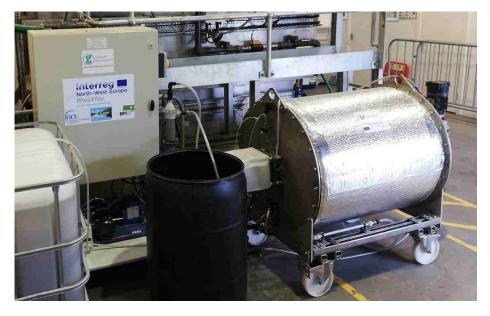
Figure 3.5.1: 500L Photobioreactor (PBR) implemented at the Wastewater Development Centre in Bo'ness (Escudero et al. 2021)
