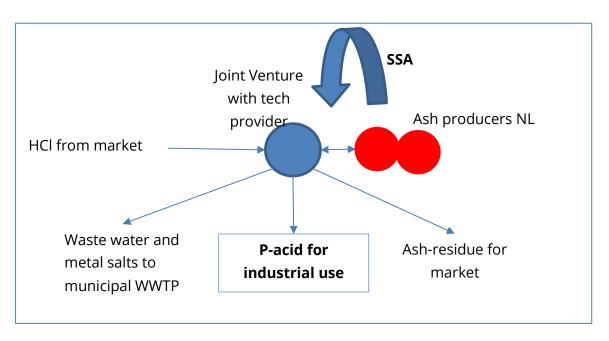
Figure 5.2.5: Schematic representation of the scenario "co-investment in P-recovery facilities to produce phosphoric acid out of sewage sludge ashes"
