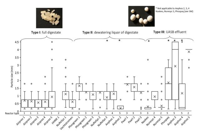
Figure 4.1.3: Mass fraction distribution per particle size for all analysed struvite samples. Crosses indicate the mean particle size (mm). Numbers indicate the reactor type as follows: 1 Airlift reactor, 2 Continues stirred tank reactor, 3 Fluidized bed reactor, 4 Tank aerated, 5 Tank mixed (Muys et al. 2021).
