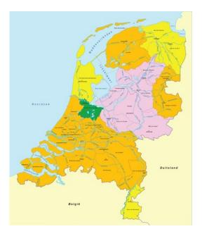
Figure 5.2.1: Sewage sludge treatment in The Netherlands (orange = incineration; pink = composting; yellow and green =drying and co-incineration) (©SNB)
