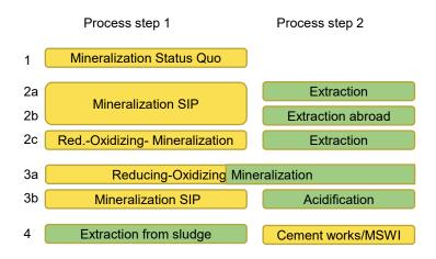
Figure 5.1.3: Illustration of scenarios for 2026 consisting of combinations of sewage sludge mineralization in yellow and phosphorus recovery in green
