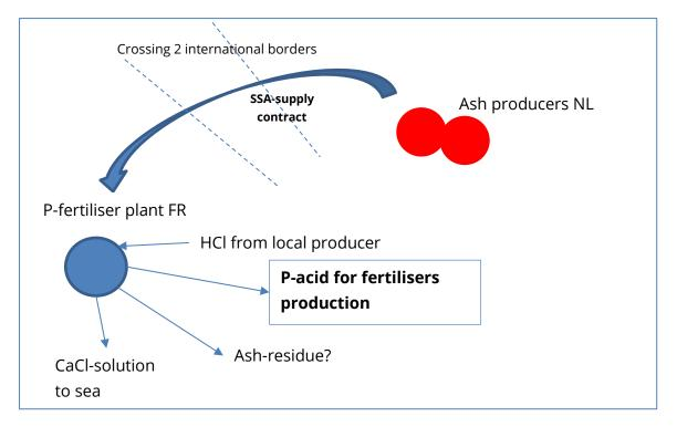
Figure 5.2.3: Schematic representation of the scenario "sewage sludge ash delivery from The Netherlands to a plant of an external provider located in France
