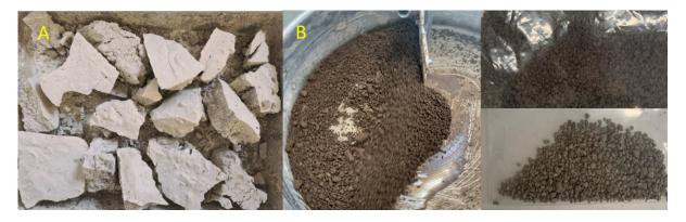
Figure 3.4.1: A - PULSE product filter cake dried; B- granulation tests on PULSE product performed by Prayon S.A (Shariff et al. 2021)
