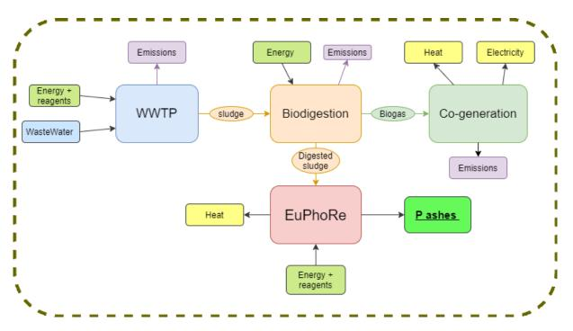
Figure 3.8.3: System boundaries for the EuPhoRe<sup>®</sup> system with the avoided burden approach (Chantrain et al. 2021)
