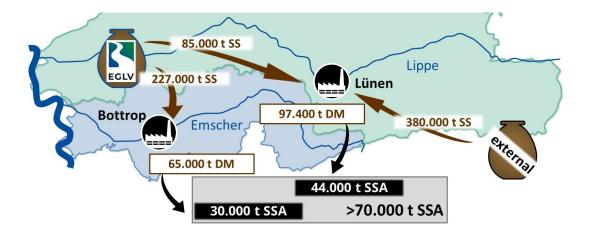
Figure 5.3.1 Perspective of the SS flows and the SSA produced at the sites of EG (Bottrop) and Innovatherm (Lünen) in 2029 (planning basis) (Blöhse et al. 2021)
