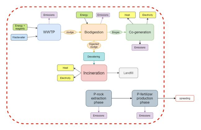
Figure 3.8.1: General boundaries for the LCA (system expansion approach) (Chantrain et al. 2021)
