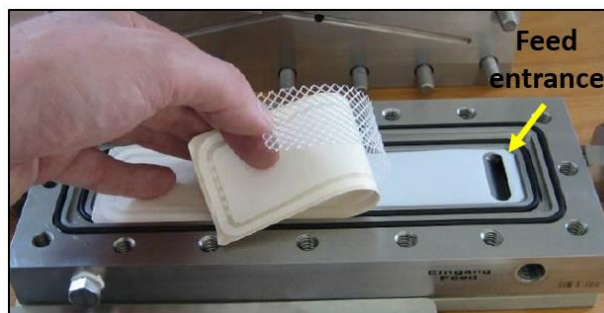
Figure 33: Construction of the spacer-filled channel.
