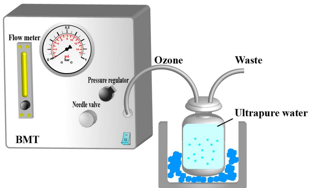
Figure 9 Setup of the ozone generator. The ozone stock solution was in ultrapure water
