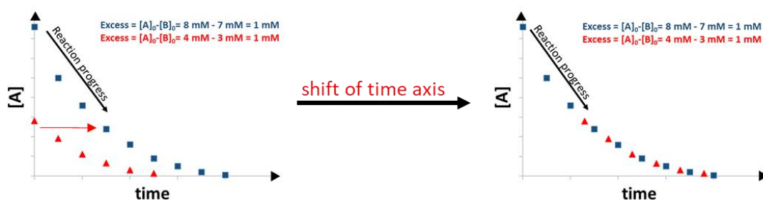
Figure 39: Same excess experiments to check for catalyst deactivation/product inhibition. Addition of a value S to the time axis of the red curve results in overlay of both conversion curves.
