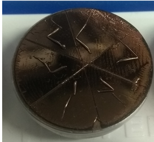
Figure 4.2: Prepared scanning electron microscope sample. Double sided tape is stuck to the sample holder and slices for the legs marked. The dried and dissected legs are placed and the whole holder is sputtered with gold.
