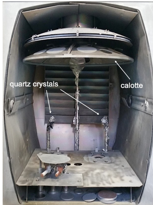
Fig. 18: Balzers Process Systems BAK 640 coating system high vacuum chamber, with a calotte and quartz crystals.
