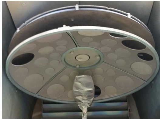
Fig. 20: Rotatable calotte used as a substrate holder.
