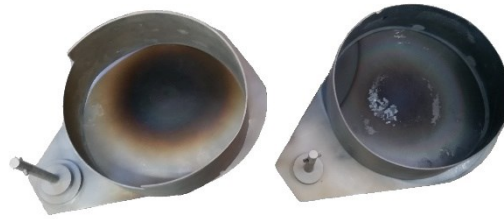
Fig. 19: Crucibles to be filled with self-made Ti_2O_3 or Nb_2O_5 pellets.
