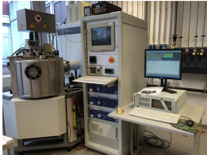
Fig. 23: Von Ardenne Anlagentechnik GmbH LS500s sputter coater equipped with a PEM. 106
