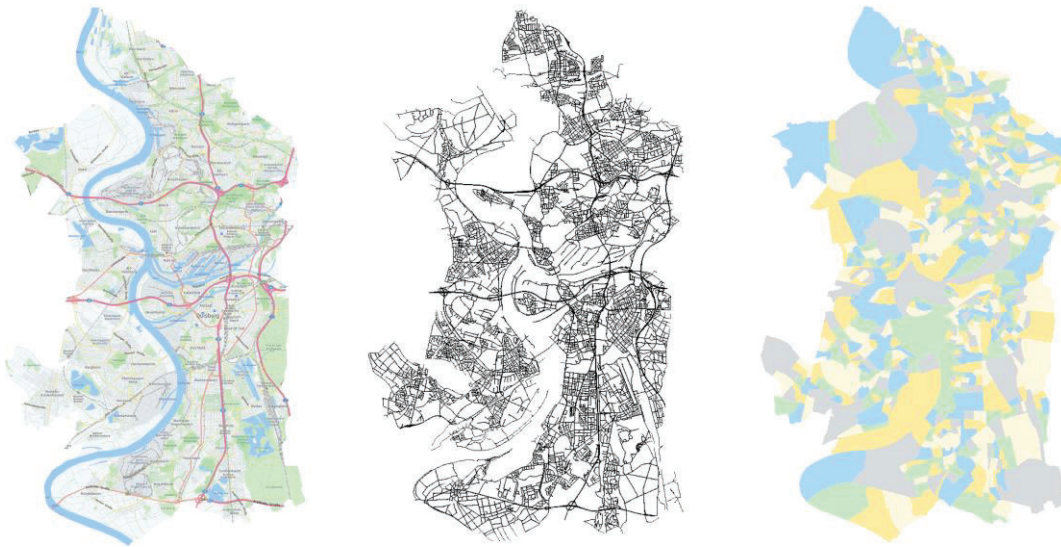
Figure 3.10: Map, extracted network and OD matrix partition of the city of Duisburg.
