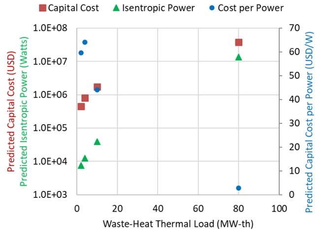
**Figure 13:** Capital cost and power output predictions for various thermal scales
