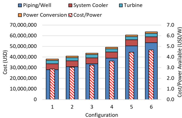
**Figure 12:** Capital cost predictions for 80 MW-th geothermal application
