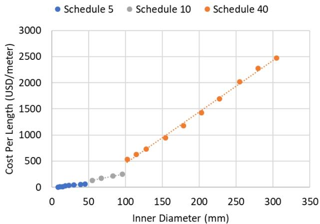
**Figure 4:** Linear cost function, pipe schedule selected using ASME B31.1 power piping code.
