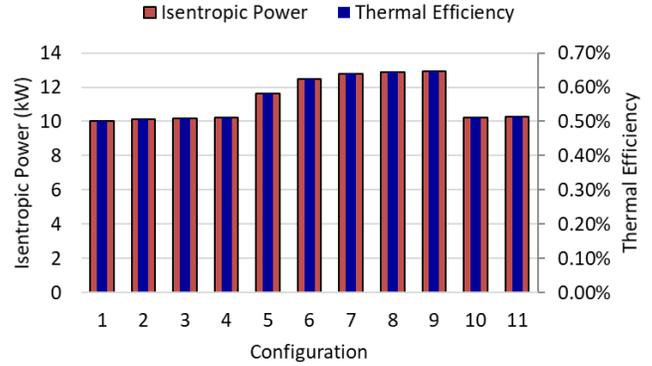
**Figure 7:** Cycle performance predictions for 4 MW-th data center
