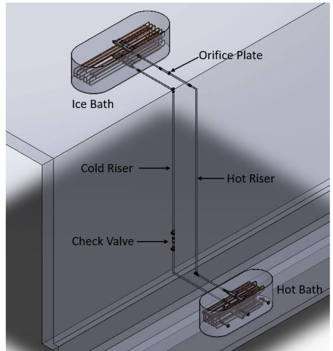
Figure 2: Lab-scale natural convection test loop
