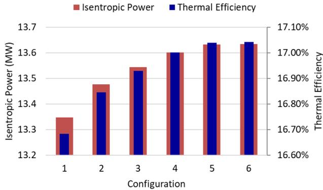
**Figure 11:** Cycle performance predictions for 80 MW-th geothermal application
