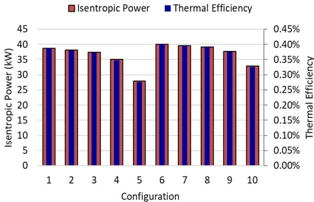
**Figure 9:** Cycle performance predictions for 10 MW-th industrial application
