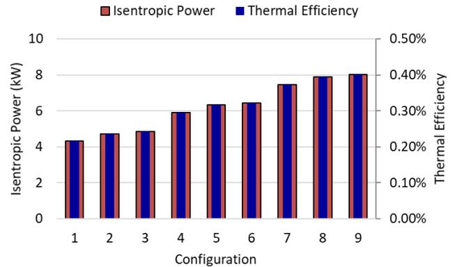
**Figure 5:** Cycle performance predictions for 2 MW-th data center
