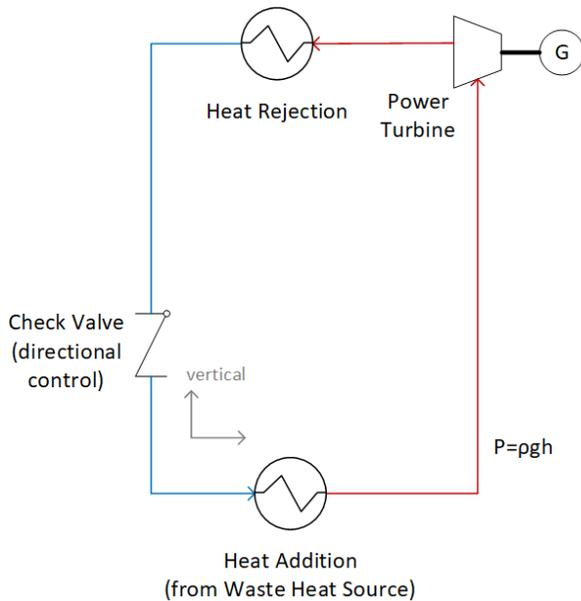
**Figure 1:** Schematic of natural convection power cycle.
