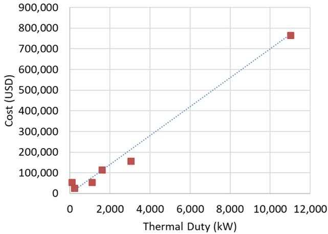
**Figure 3:** Summary of heat exchanger quotes used to define cost function.
