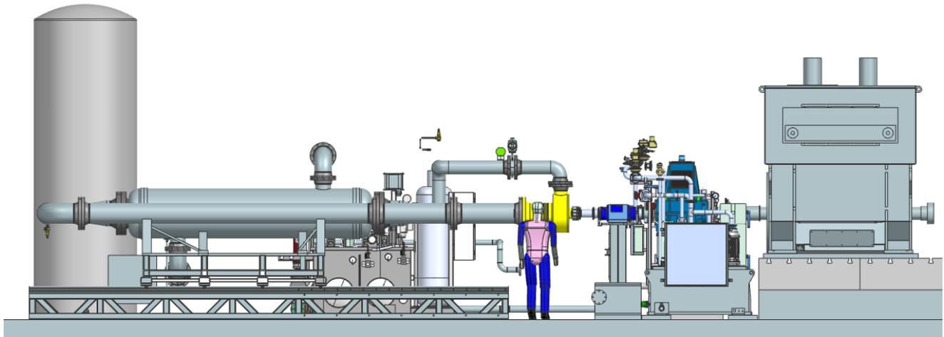
**Figure 4a:** Layout of CO<sub>2</sub> compressor test facility.
