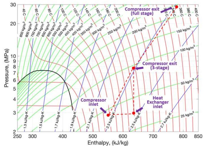
**Figure 2:**  $p$ - $h$  diagram of the 3 stage test compressor in test loop vs full stage compressor operating point.
