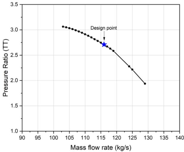
**Figure 1:** Predicted map of a 3-stage axial compressor @ design point
