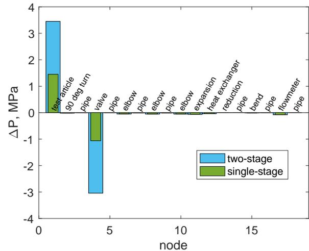
**Figure 5:** Pressure resistance of the main CO<sub>2</sub> test loop in single stage and two stage compressor configurations. Losses from the components are found to be small to allow mapping the test in single stage configuration. Most of the pressure resistance is generated through throttling at compressor exit.
