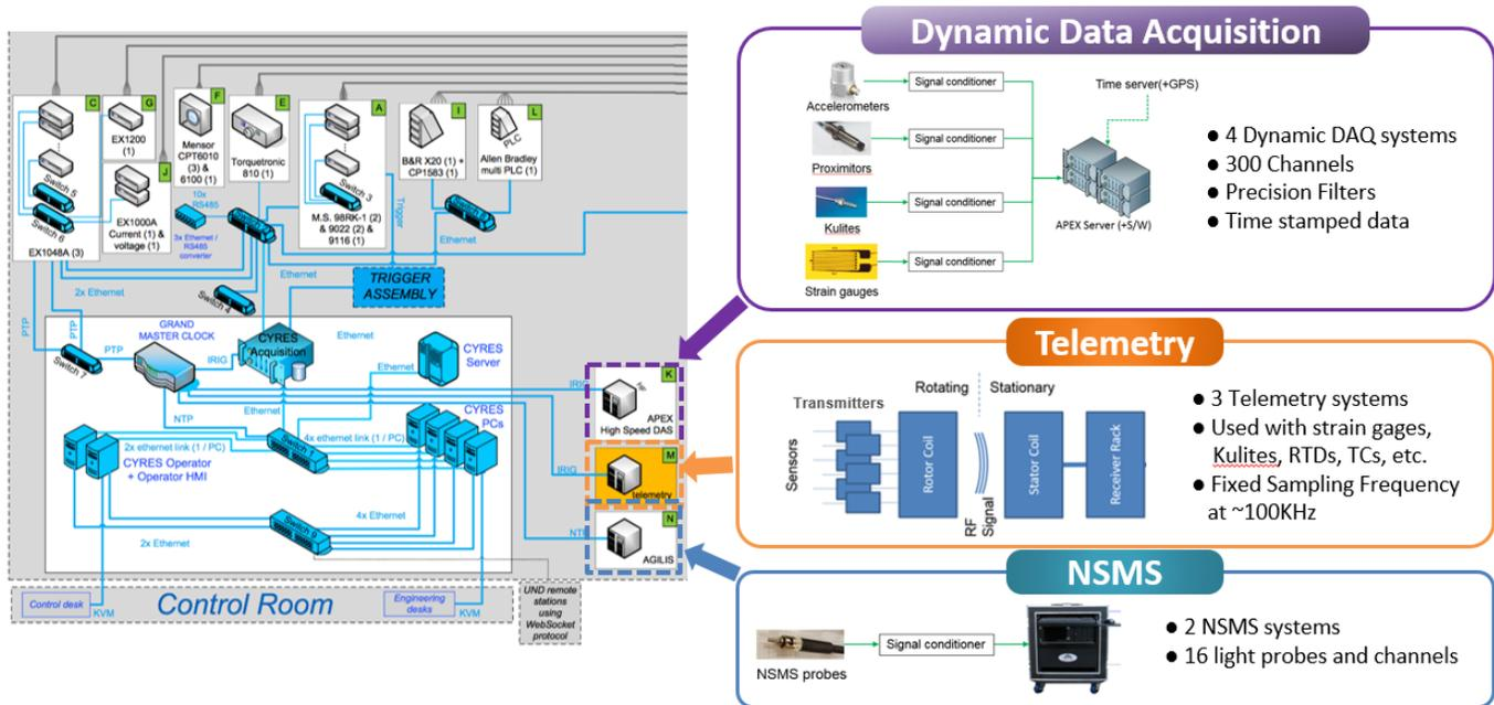
**Figure 6:** Schematic of the data acquisition system. Low speed data acquisition system for temperatures, pressures, flowrates, etc. and high speed data acquisition system for vibrations, dynamic pressures, strain gages, light probes, and the telemetry system are connected with the main facility control system.
