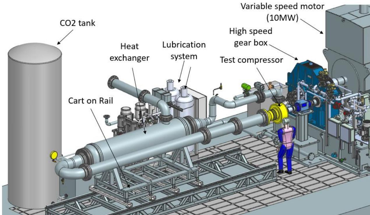
**Figure 4b:** CAD model of CO<sub>2</sub> compressor test facility. A main CO<sub>2</sub> closed loop, a CO<sub>2</sub> tank and inventory system, test rig lubrication system, and drive train (a motor, a gear box, and a torquemeter) is shown in the model.
