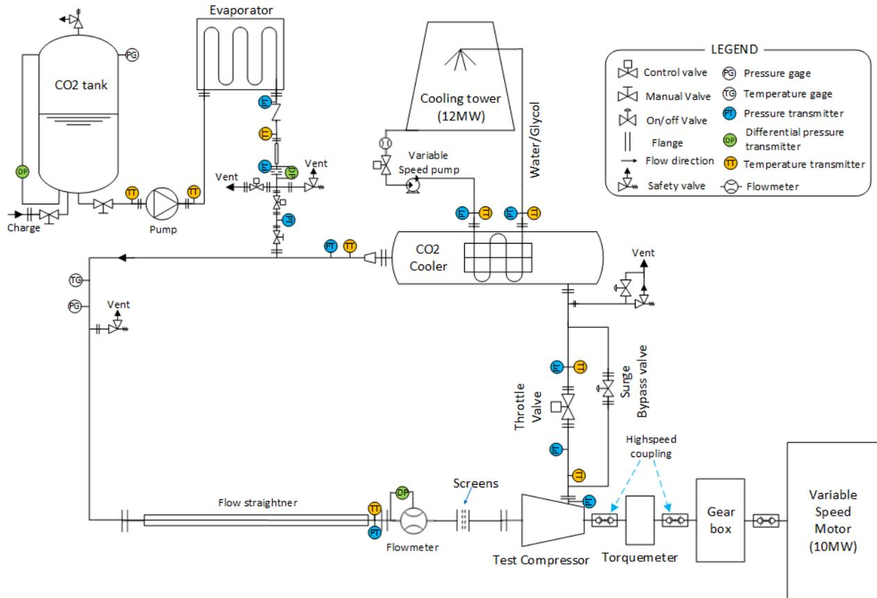
**Figure 3:** Schematic diagram of sCO<sub>2</sub> compressor test facility.
