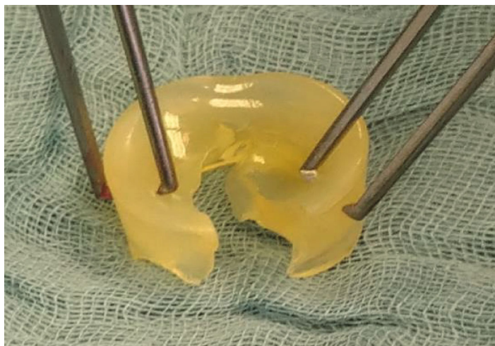
FIGURE 4: Crack in the explanted silastic radial head prosthesis after 14 years of durability.
