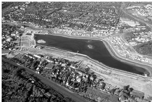
(1) Phoenix Lake in Dortmund, Germany. The lake is an example of urban integrated watershed management, where the area, a former industrial plant, was revitalized featuring a lake for flood retention, recreational and commercial areas, as well as housing. Source: Rupert Oberhäuser/EmscherGenossenschaft
