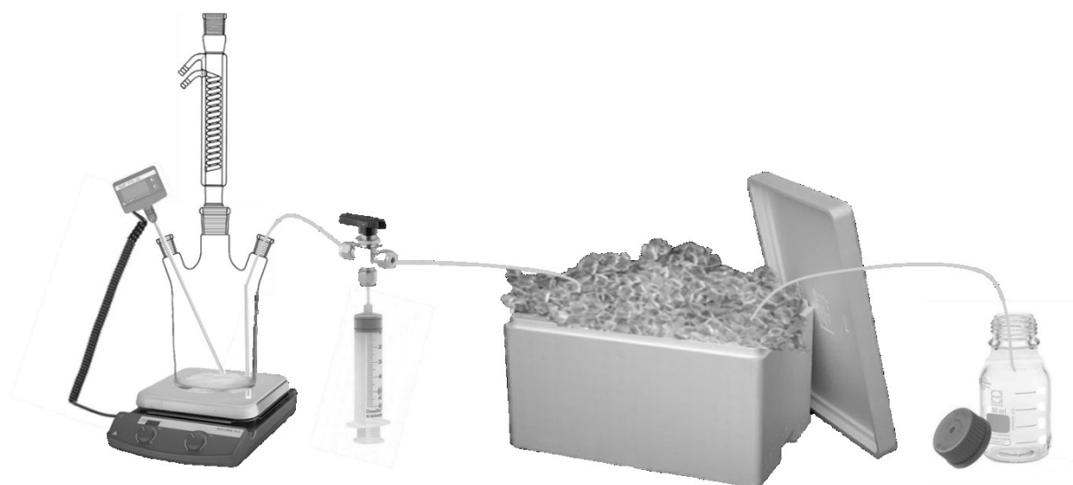
Figure 5.1: Setup for the mineralization experiments: triple-necked glass flask with reflux cooler, heating plate with automatic temperature control, manual three-port valve, and crushed ice cooling system
