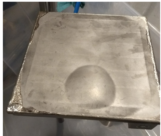
Figure 10: Photograph of coversheet bulge failure.
