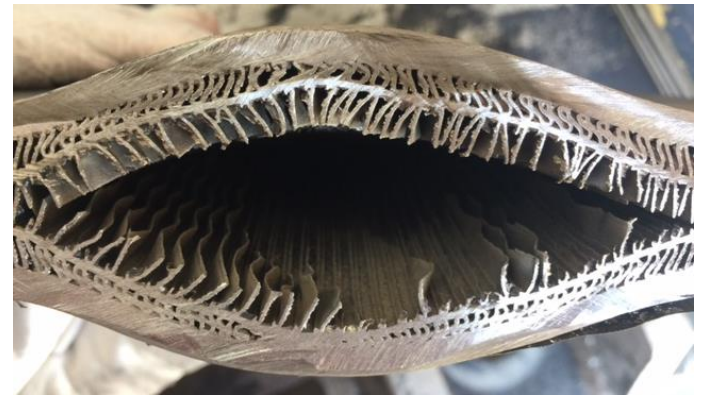
Figure 7: View of the rupture location of a brazed sample composed of "square"-shaped fins
