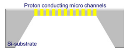
Figure 15: Silicon micro MEA based on a free-standing membrane with uniform array of micro channels.
