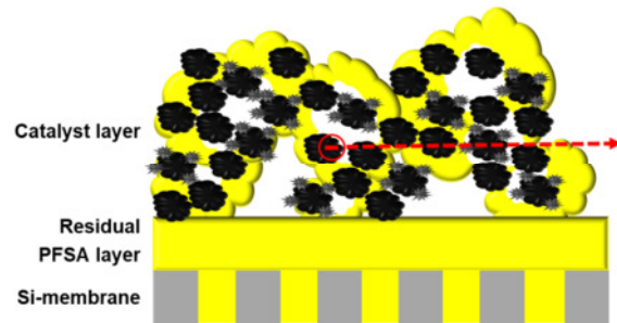
Figure 80: Theoretical pathway of an electron at the anode of a silicon-based \mu MEA. As no gas diffusion layer is used, electrons have to be conducted through the catalyst layer in horizontal direction.
