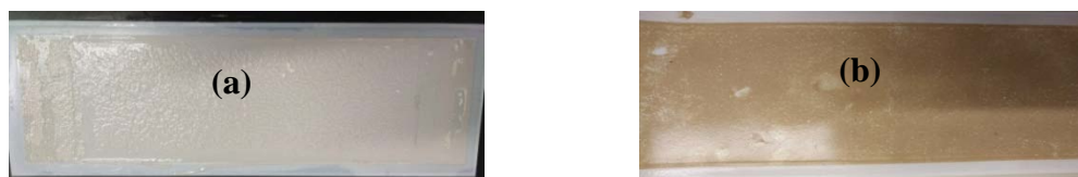
Figure 2. UP005P membrane morphology: (a) 1:500 dilution FS and ZnO, (b) 1:500 dilution FS
