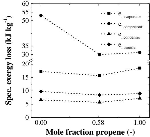
Fig. 11: Specific exergy loss of each component as a function of the propene mole fraction for  $n = 1050 \text{ min}^{-1}$  without the approach to minimize the exergy loss (case 3).
