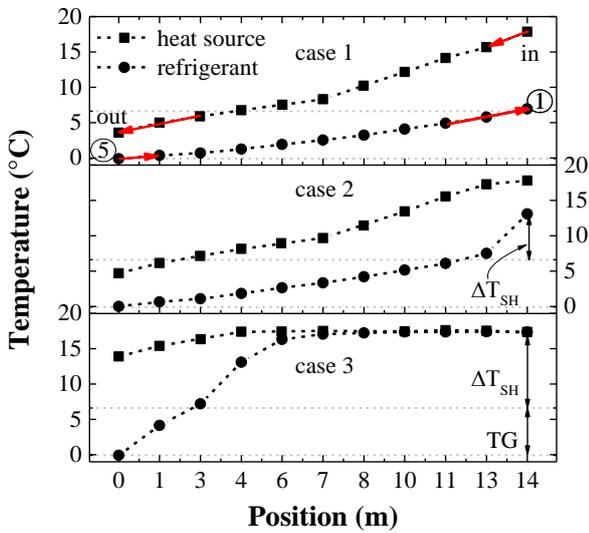
Fig. 3: Temperature profile of the refrigerant and the heat source in the evaporator as a function of evaporator length for  $T_L = 0 \text{ }^\circ\text{C}$ ,  $n = 1050 \text{ min}^{-1}$  and three different heat capacity flows.
