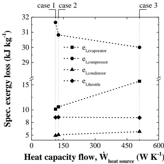
Fig. 5: Specific exergy loss of each component as a function of the heat source capacity flow for  $n = 1050 \text{ min}^{-1}$ .
