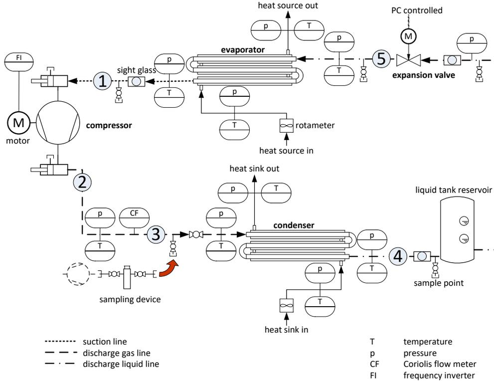
Fig. 1: Schematic flowchart of the experimental rig.
