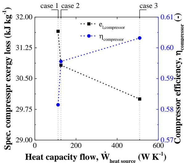
Fig. 8: Specific exergy loss and the global compressor efficiency of the compressor as a function of the heat source capacity flow for  $n = 1050 \text{ min}^{-1}$ .
