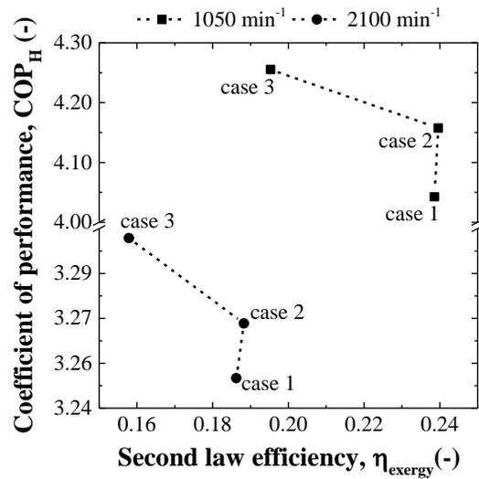
Fig. 6: Coefficient of performance as a function of the exergetic efficiency for investigated scenarios;  $n = 1050 \text{ min}^{-1}$  and  $n = 2100 \text{ min}^{-1}$ .
