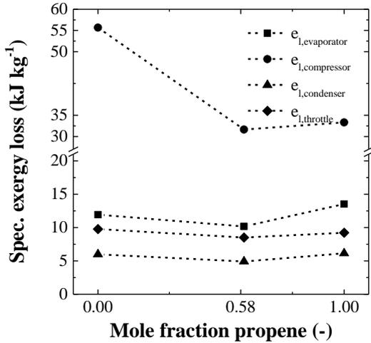
Fig. 10: Specific exergy loss of each component as a function of the propene mole fraction for  $n = 1050 \text{ min}^{-1}$  with the aim of minimizing the exergy loss (case 1).
