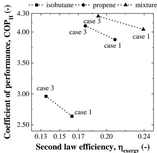
Fig. 12: Coefficient of performance as a function of the second law efficiency for  $n = 1050 \text{ min}^{-1}$  for isobutane, propene and the mixture with respect to lowest and highest exergy loss scenario.
