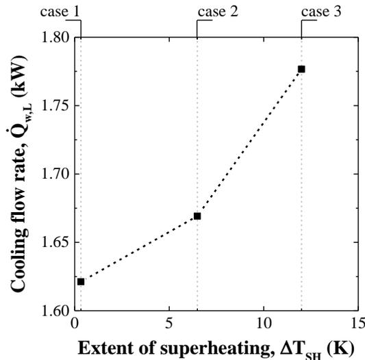
Fig. 7: Evaporator cooling flow rate as a function of superheating for  $n = 1050 \text{ min}^{-1}$ .
