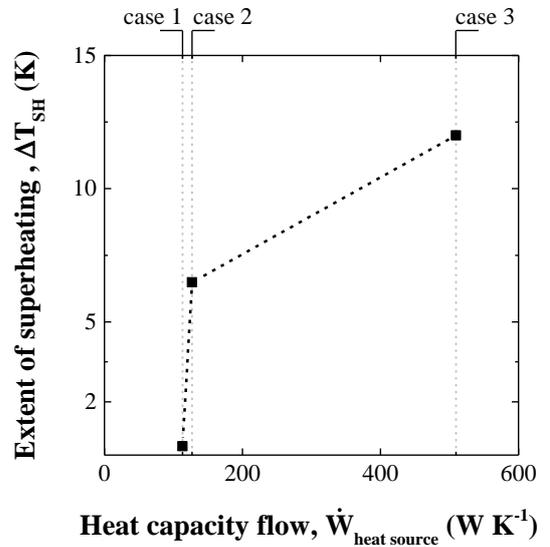
Fig. 4: Attained superheating of the refrigerant as a function of heat capacity flow for  $T_L = 0 \text{ }^\circ\text{C}$ ;  $n = 1050 \text{ min}^{-1}$ .
