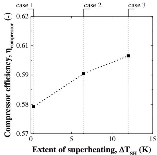
Fig. 9: Compressor efficiency as a function of the extent of superheating for  $n = 1050 \text{ min}^{-1}$ .
