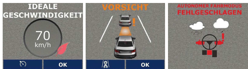
(b) Fuel efficiency suggestion in SEMI driving mode
