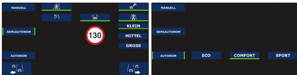
(c) SEMI driving mode with activated vehicle-following function
