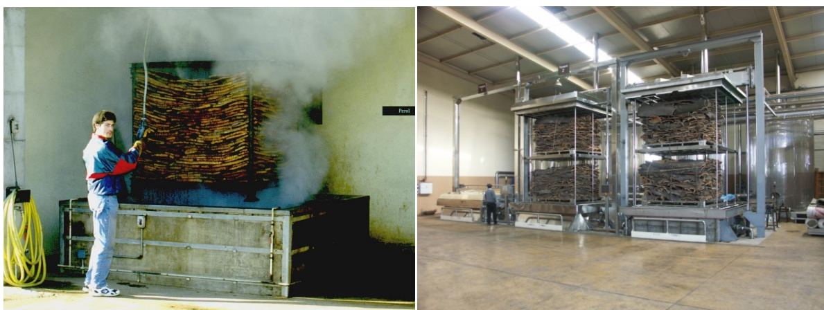
Figure 1-4 Traditional (left) and modern (right) water boiling process of cork planks (photo: Rudolf Ohlinger GmbH)
