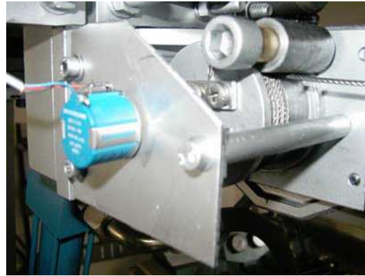
(b) Rotary potentiometer for L(t)
