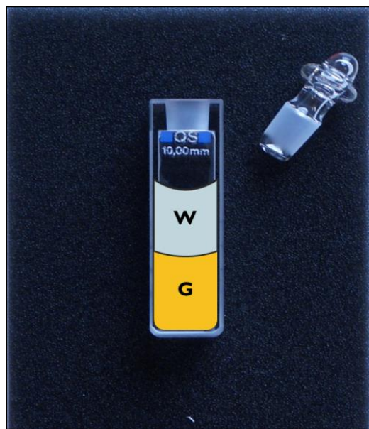
Figure 19 The experimental system used to evaluate the partitioning of phenanthrene between polysaccharide gels and water. The gel solution (G) was poured into the QS glass cuvette and the deionized water solution of phenanthrene (1.5 mg/L) was added above (W). Also the glass stop is shown in the picture on the left side.
