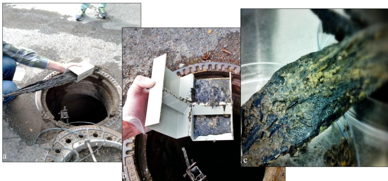
Figure 13 Overview of the devices used for sampling sewer biofilms. a, b) the biofilm is scratched off from the sampler into a special tool. c) a closer look at the sewer biofilm attached on the PFT support used for the sampling procedure.
