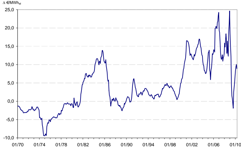
Fig. 4.5: Differences in total operating costs of new CCGT and hard coal plants in Germany 1970–2010 (source: BAFA (2010); StaBu (2010); EEX (2011); own analysis).
