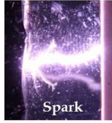
Figure 38. Image of a spark discharge ( \sigma = 0.1 \mu\text{S/cm} , U = 30 \text{ kV} , d = 1.4 \text{ cm} , camera gate width is 1 \text{ s} ). The image size is 13.5 \times 16 \text{ mm}
