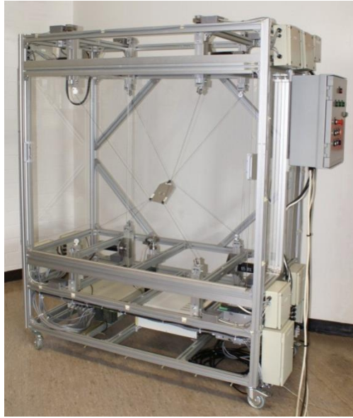
Figure 3.2: The Segesta Cable Robot [32].
