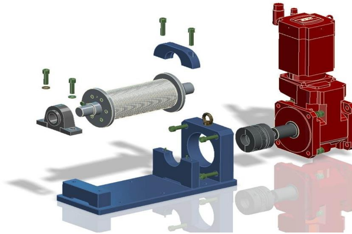
Figure 6.2: Installation of the Cable Cylinder Machine with motor [48].
