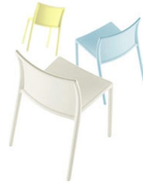
Figure 16. The “Air Chair”, designed by Morrison, is a successful design which derives from the properties of composite “polypropylene” and the gas-injection technology that is used to manufacture it. The properties of the composite alone are too flexible to create the chair, so, before molding it, it is mixed with fiberglass to add strength. Morrison relates this highly technological process to natural principles by describing the chairs as being ‘like a bone’ [Morrison, 2002].
