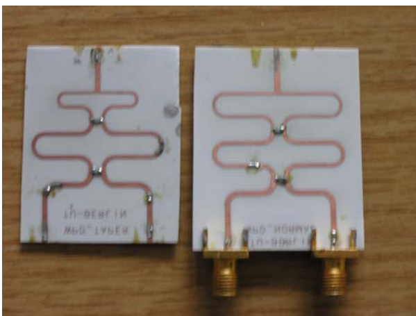
Figure 3. Photograph of the realised combiners; tapered on the left, normal on the right side.
