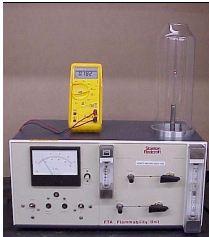
Abbildung 4.2 LOI-Messinstrument "FTA Flammability Unit" der Firma Stanton Redcroft
